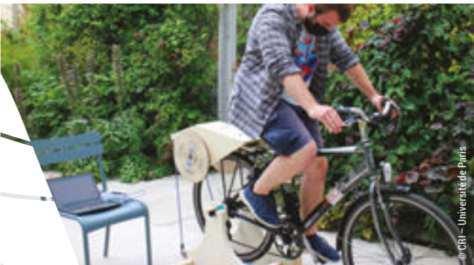
Prototype of a frugal centrifuge for use in low-income biology labs
